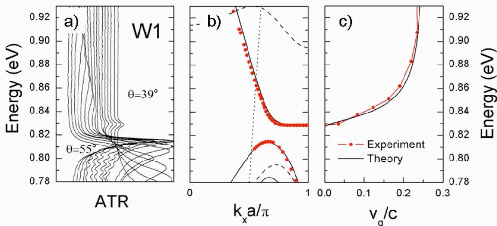
Figure 2. (a) Experimental ATR spectra measured on a single line-defect W1 waveguide, for TE polarization (curves are shifted for clarity). (b) Measured dispersion of the photonic bands as derived from ATR spectra (closed circles) compared to calculated dispersion (lines). (c) Experimental group velocity dispersion (closed circles) compared to calculated dispersion (line).
