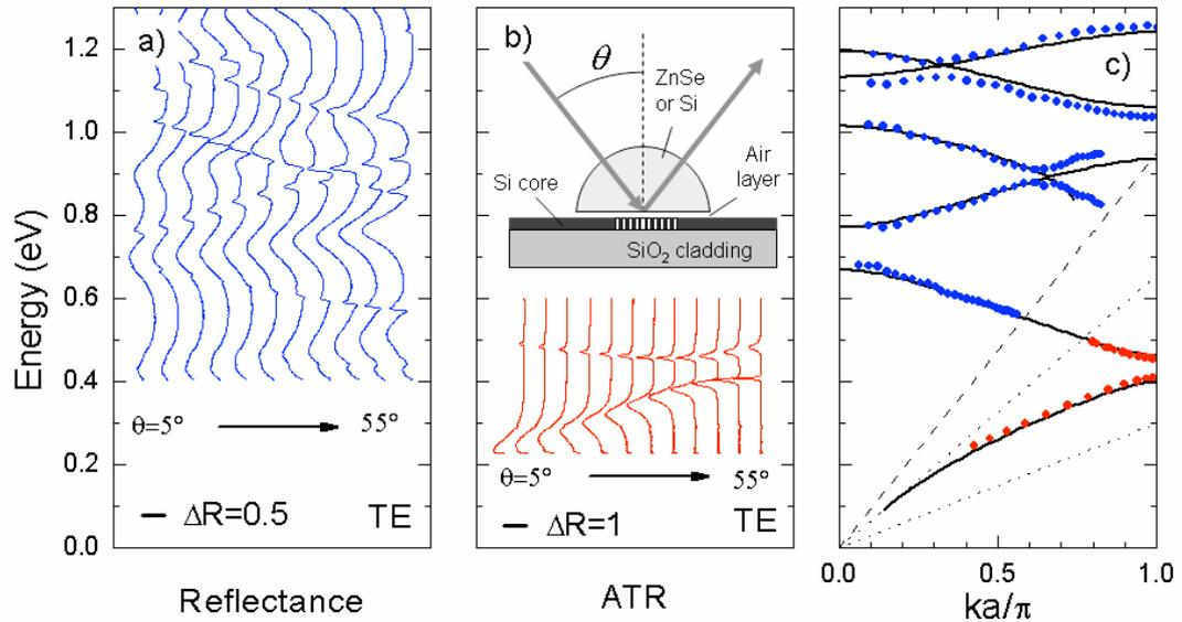
Figure 1. Experimental reflectance (a) and ATR (b) spectra for the 1D SOI PhC sample measured for TE polarization (curves are shifted for clarity). (c) Dispersion of the photonic bands as derived from reflectance and ATR spectra, compared to calculated dispersion (lines). Dotted lines: light lines of air, SiO<sub>2</sub> and Si.
