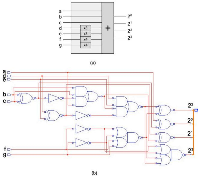
Figure 5. Cell 1112244: symbol (a) and circuit (b).
