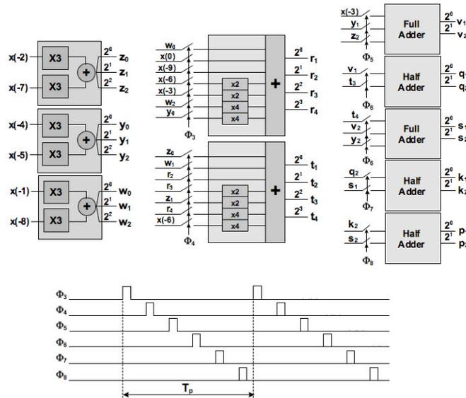
Figure 8. Proposed  $\text{sinc}^3$  filter: pipeline approach.
