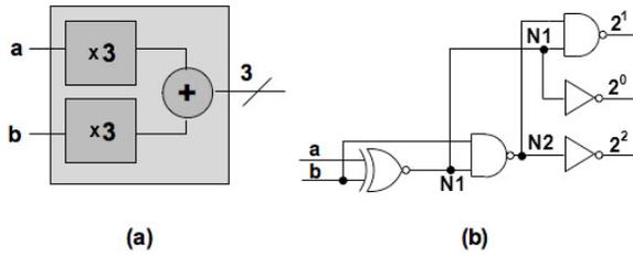
Figure 3. Cell 33: symbol (a) and circuit (b).
