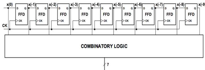
Figure 1. A  $\text{sinc}^3$  conventional design.
