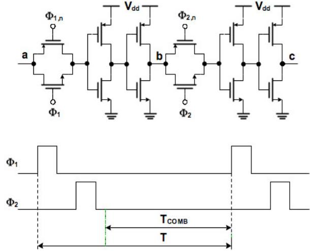
Figure 2. Delay line cell and its control signals.
