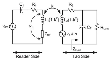
Fig. 1. Equivalent circuit of magnetically coupled power link
