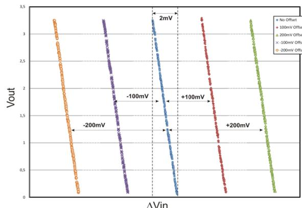
Figure 7:  $V_{out}$  variation after calibration for a maximum of  $\pm 200mV$  as differential input offset.
