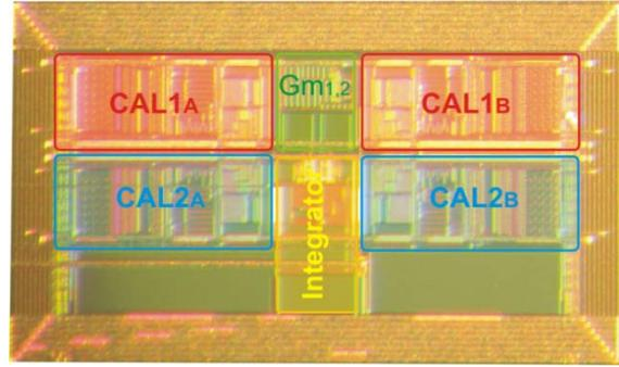
Figure 5: Microphotograph of the implemented readout circuit.
