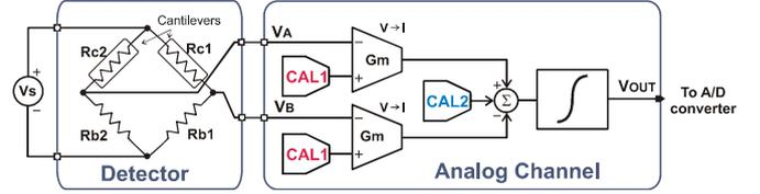
Figure 2: Simplified schematic of the readout channel.
