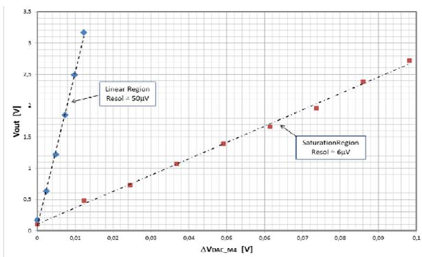
Figure 6:  $V_{out}$  variation depending on the fine calibration input values.
