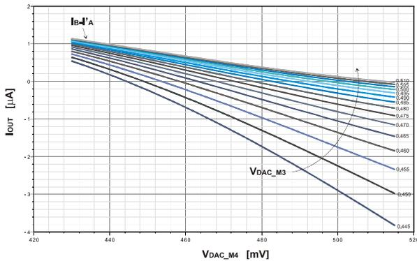
Figure 4: Current variation of  $I_{OUT}$  depending on  $V_{DAC\_M4}$  for different values of  $V_{DAC\_M3}$ .
