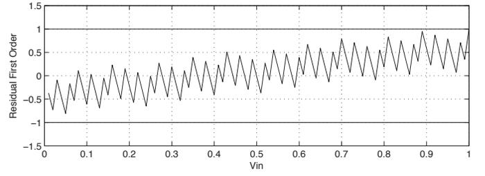
Fig. 4. Range of the residual for a single channel first order of time-interleaved incremental as function of the input amplitude.
