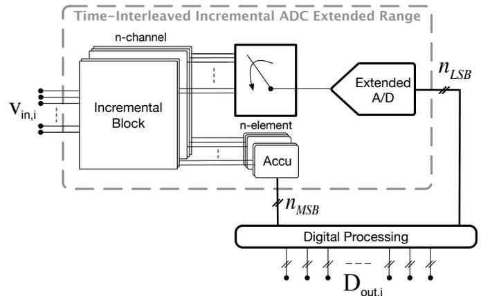
Fig. 1. Proposed system level diagram of multichannel time-interleaved incremental ADC (TIADC) with extended range A/D.
