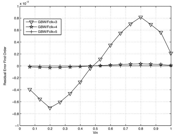
Fig. 7. Residual errors caused by slew-rate and bandwidth for the first order scheme.
