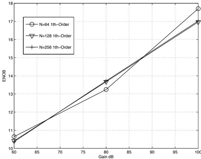
Fig. 6. Maximum achievable ENOB with an extended range incremental converter for a given op-amp DC gain.
