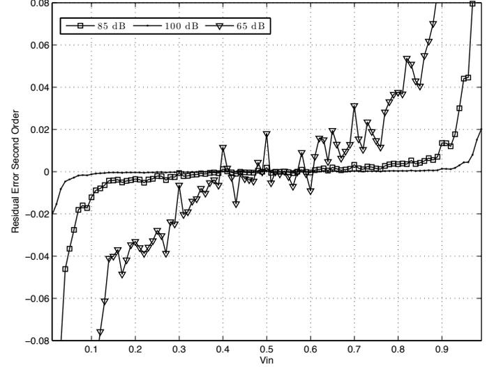
Fig. 5. Residual error of a first order converter as a function of the input amplitude for different op-amp gains.
