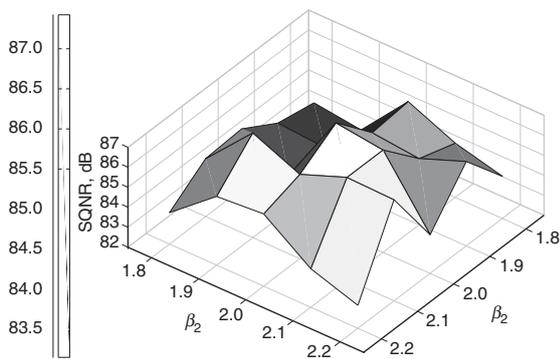
Fig. 5 SQNR against gain of auxiliary amplifier for first ( $\beta_1$ ) and second ( $\beta_2$ ) integrator
