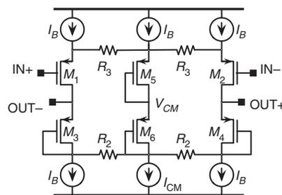
Fig. 2 Simple amplifier with accurate gain
