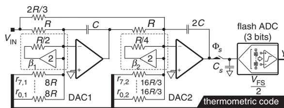
Fig. 3 Second-order gain-compensated CT  $\Sigma\Delta$  modulator
