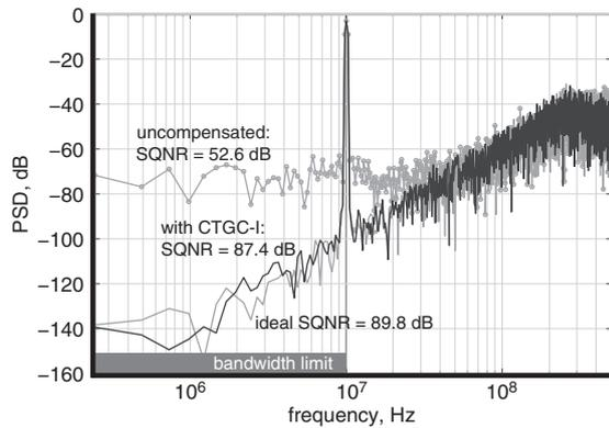
Fig. 4 Power spectral density comparison, 4096 FFT points
